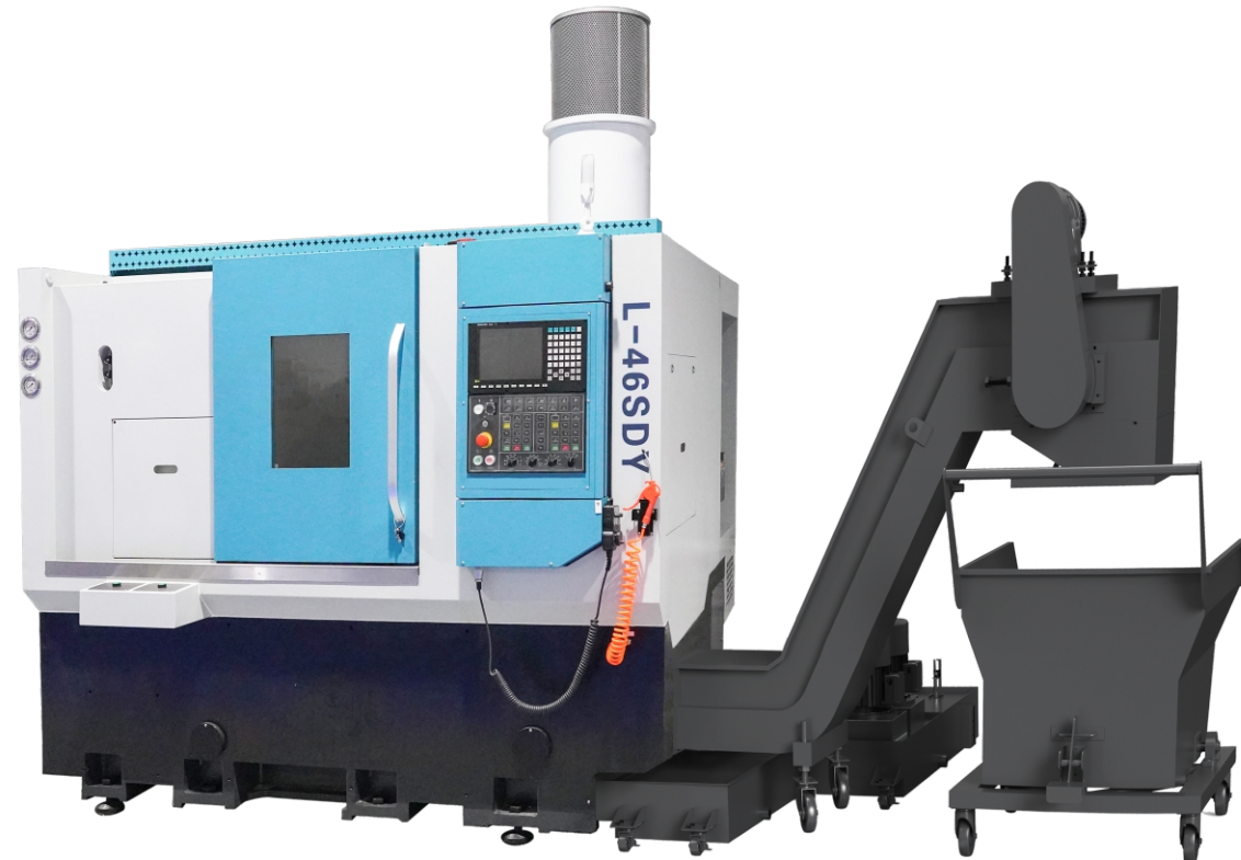
Characteristics of the 30° integrated bed structure Perfect rigidity and stability
