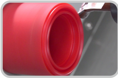
Turning sealing profiles with professional cutting edge
