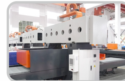
Gantry fixed beam structure
