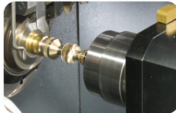
Sub-spindle butt joint workpiece with main spindle.
