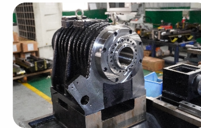
Large torque with belt type spindle
