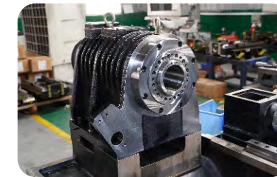
Large torque with belt type spindle
