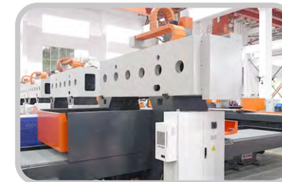
Gantry fixed beam structure
