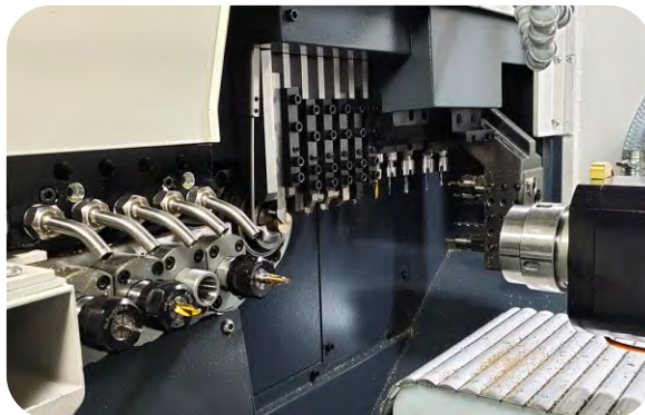
ST-265 Standard tool holder with 20 pcs Main and sub-spindle with two-channel control.
