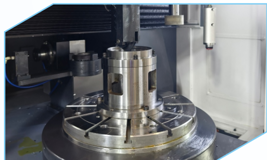
Grinding Inside gear profile
