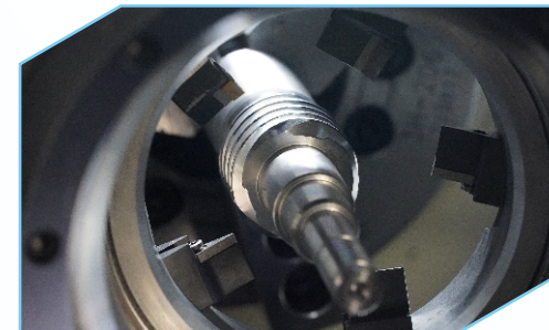
Surface roughness Ra 0.4-1.0 μm after milling
