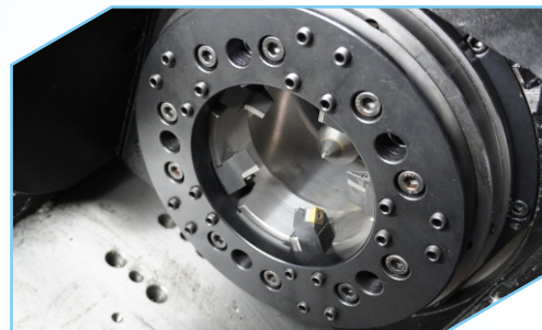
Internal whirling with 5- insert
