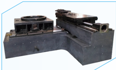
Mixed mineral base stands with low expansion coefficients
