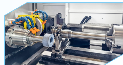
Working table swing angle +30/0°by manual
