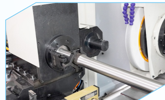
The rigid constructed spindle head with reducer to get large torque
