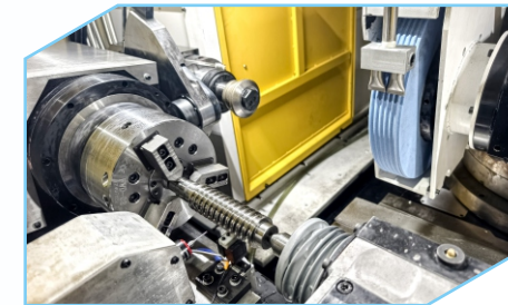
Forming wheel with rapid grinding
