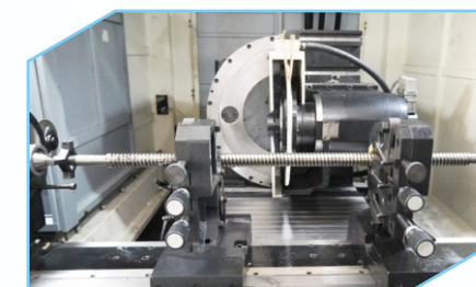
Steady rest for support long workpiece
