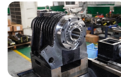
Large torque with belt type spindle
