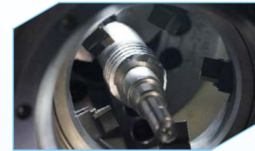
Surface roughness Ra 0.4-1.0um after milling
