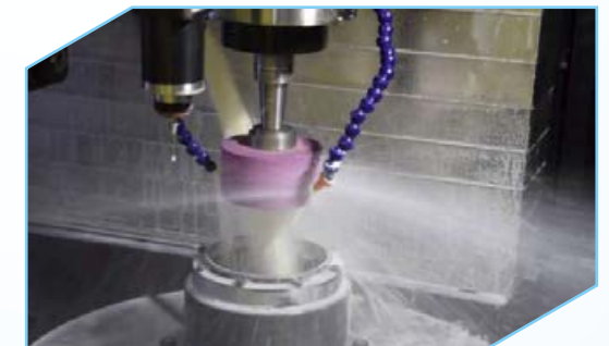
Internal grinding process
