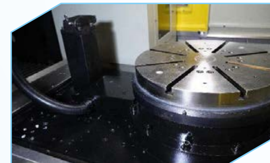
Turntable with grating scale to improcvce precision
