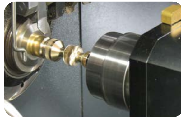
Sub-spindle butt joint workpiece with main spindle.
