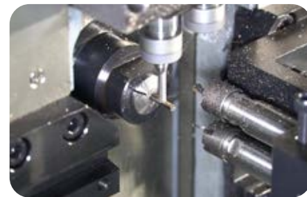
2pcs live tool on Y axis 8pcs turning tool 3 pcs front drilling tool
