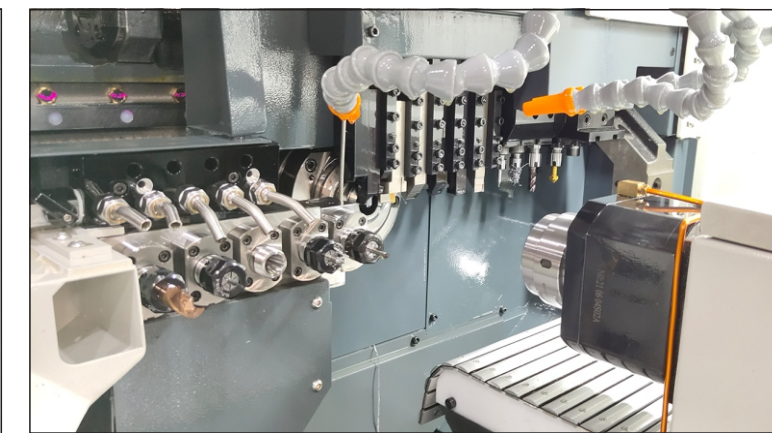
ST-265 standard tool holder with 20 pcs (Optional adding 2pcs rotary tools on back spindle ) ;Main and back spindle with two-channel control.
