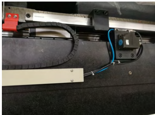
Digital scales and encoders, supported by a sturdy base and prismatic guide
