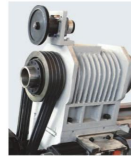
smooth rotation of the spindle after dynamic balance process
