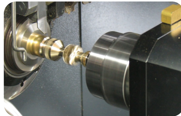
Sub-spindle butt joint workpiece with main spindle.
