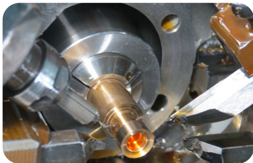
The inner and outer diameters of workpiece can be processed simultaneously.
