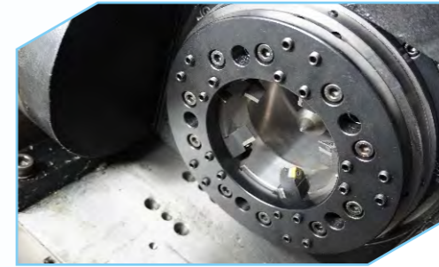
Internal whirling with 5- insert
