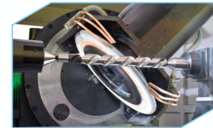
Grinding wheel leadangle +20° -160°
