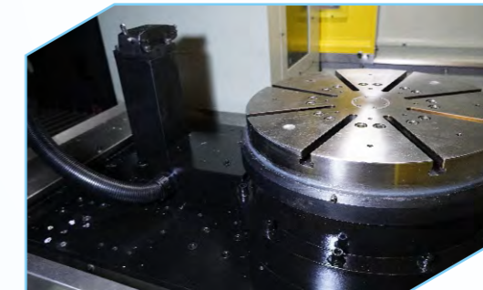
Turntable with grating scale to improve precision
