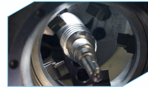
Surface roughness Ra 0.4-1.0um after milling
