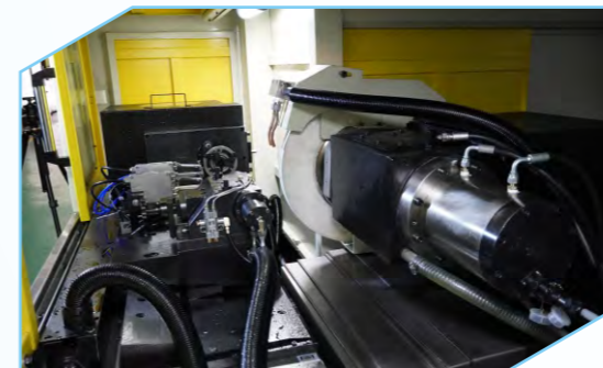
Dynamic and hydrostatic grinding wheel spindle
