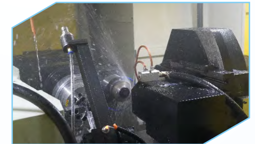
X axis and Z axis will interpolation dressing together.
